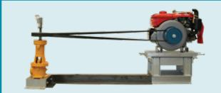
NOTE: Safety guards have been removed for display purposes. Mono Pumps supply and recommend safety guards be used on all vee-belt drive arrangements.
